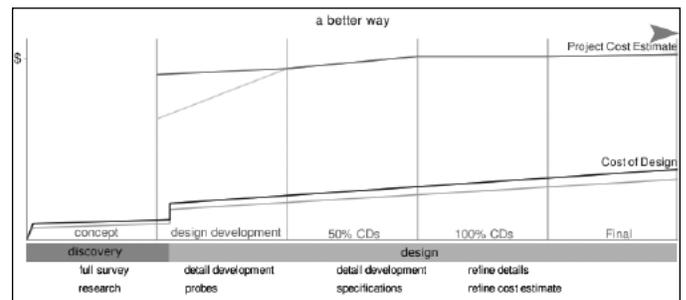
Fig. 2. Cost vs. time graph for a project for which a full survey is completed during discovery.
